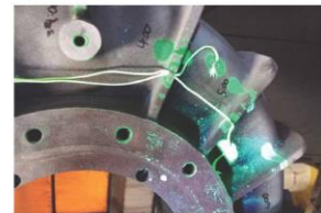
Cracks after initiating at burner rig test of turbocharger turbine casing
