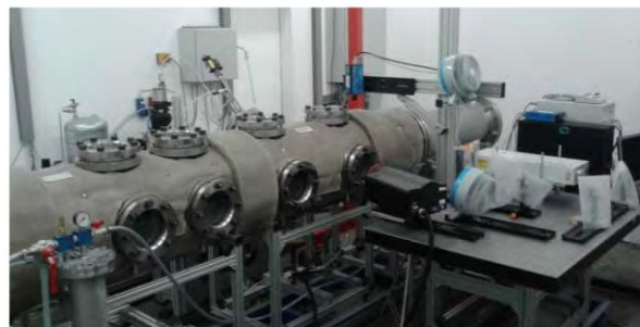
Hot exhaust gas flow rig for investigation of urea injection, evaporation and mixing
